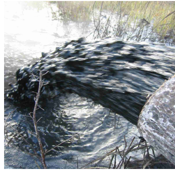
Thick mixture coming from the dredger to the 1st sedimentation pond
