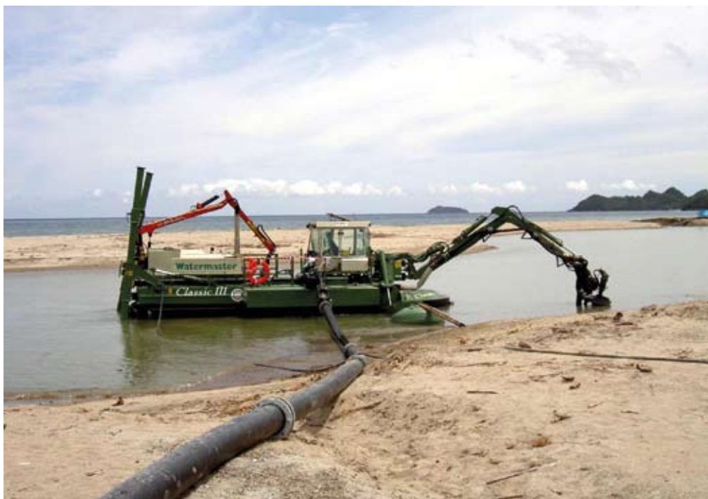
Watermaster Classic III, a Finnish made multipurpose dredger.
